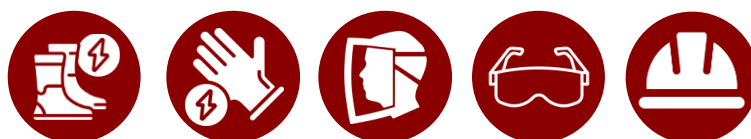
Exhibit 69 Appropriate personnel safety gear while working on High-Voltage Equipment
